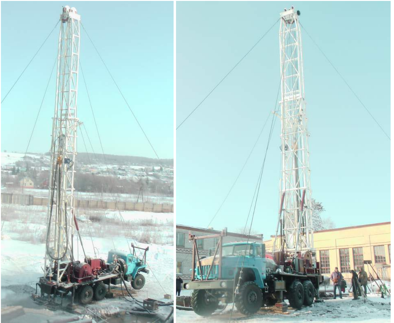
Drilling rig URB-40 onto the URAL-4320 chassis
